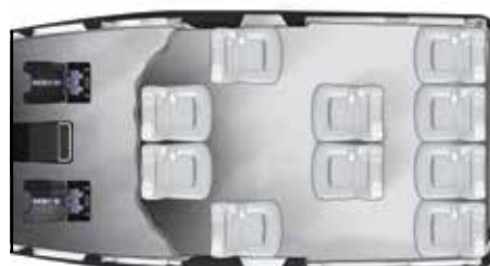
Layout - 5 (10 Passengers + Curtain) No Separation Wall Available
