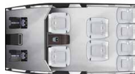
Layout - 4 (8 Passengers + FWD Cabinet + Separation Wall)
