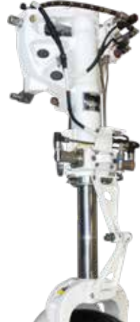
Nose Landing Gear Struts, Hydraulic Steering
